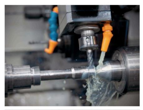
PPC engineers have developed a patented live tool design for turret lathe applications that utilizes a continuous flow of filtered machine coolant to lubricate and cool the bearings, eliminating many of the existing failure modes.
